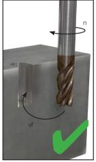
Fig. 9 Direct entering into material and entering by arc ("rolling in")
