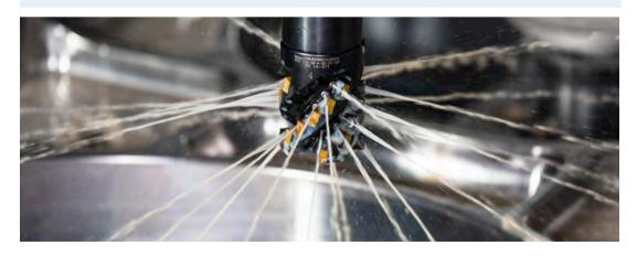
In view of this, the up-to-date machining centers, which MTB companies offer to producers of titanium components, are suitable for HPC supply. As practice shows, machining with HPC can even double cutting speed in comparison with classical As shown in practice, Accurate value for increasing cutting speed depends on specific factors. To estimate initial cutting speed in milling with HPC VHP, it is recommended to use the following equation (8):
